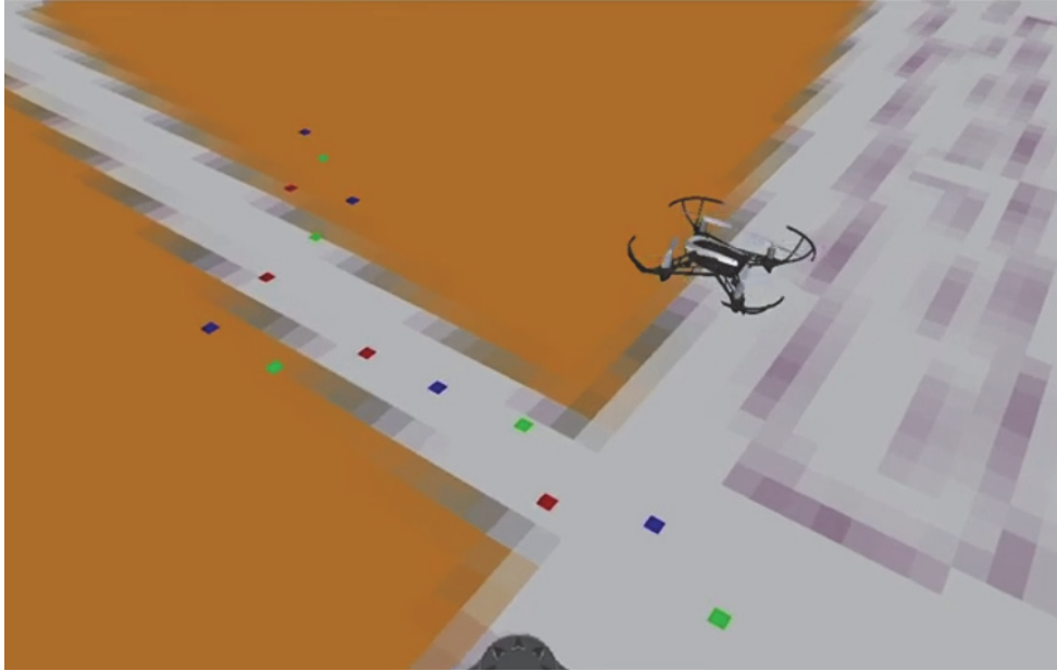
Figure 2. Competition simulator running the baseline solution (based on the Simulink Support Package for Parrot Minidrones)
